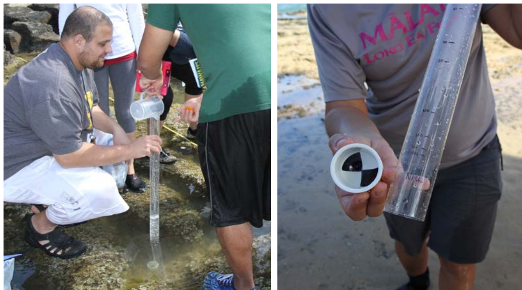
(A) (B) Fig. 4.6. (A) Researchers use a turbidity tube to measure water clarity. (B) A turbidity tube is composed of a clear tube, a stopper/cap to seal one end, a viewing disc, and a measuring device.
